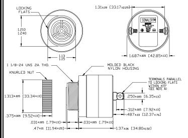
NOTE A: TERMINALS-.032 BRASS TIN PLATED, TAPPED FOR #6-32 SCREW. TWO #6-32 NICKEL PLATED BRASS SCREWS INCLUBED. WILL ACCEPT 1/4\* QUICK CONNECT. NOTE B: MOUNTING- REMOVE BLACK PLASTIC NUT AND INSERT THREADED FRINT THROUGH 1.25' HOLE PUNCHED IN PANEL, IF DRIENTATION IS NEEDED, NOTE LOCKING FLATS ON DRAWING. SCREW NUT BACK ON. DO NOT DVERTIGHTEN.
