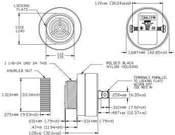
NOTE A: TERMINALS-032 BRASS TIN PLATED, TAPPED FOR #6-32 SCREW. TUD #6-32 NICKEL PLATED BRASS SCREWS INCLUBED. WILL ACCEPT 1/4\* QUICK CONNECT. NOTE B: MOUNTING- REMOVE BLACK PLASTIC NUT AND INSERT THREADED FRONT THROUGH 1.25' HOLE PUNCHED IN PANEL, IF DRIENTATION IS NEEDED, NOTE LOCKING FLATS ON DRAWING. SCREW NUT BACK ON. DO NOT OVERTIGHTEN.
